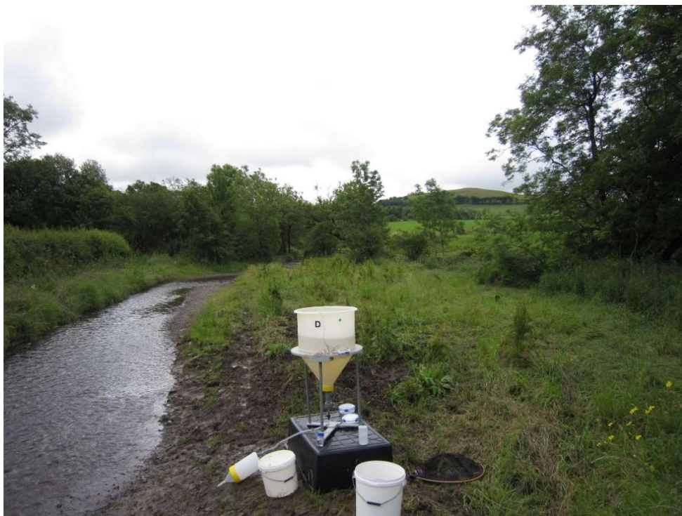
Figure 1. Equipment used in a novel non-destructive method for sampling wild salmonids for gyrodactylids
