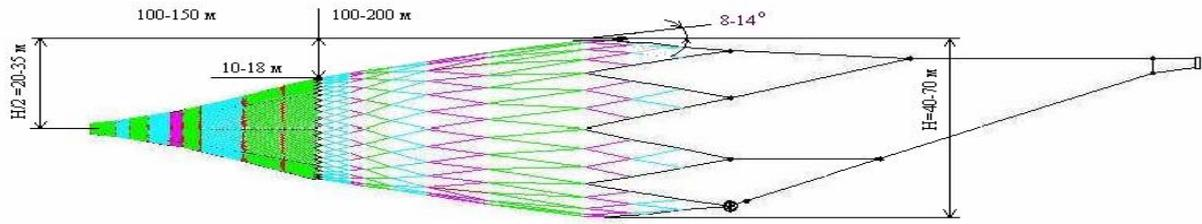
Figure 3.2.3. Schematic diagram of commercial pelagic trawl used by the Russian fleet.
