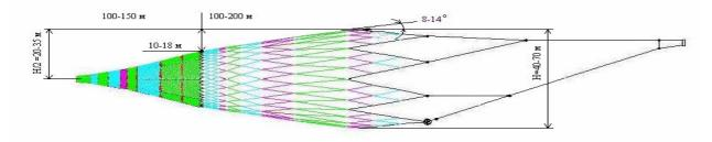
Figure 3.2.3. Schematic diagram of commercial pelagic trawl used by the Russian fleet.
