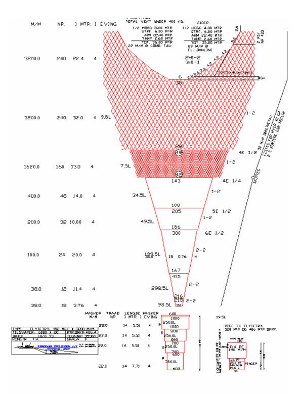
Figure 3.2.2. Pelagic species survey trawl used by IMR.
