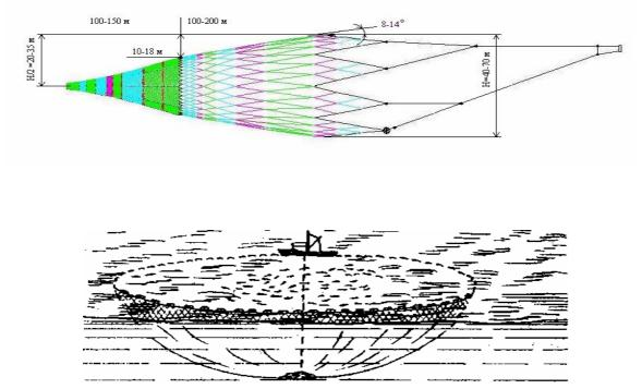
Figure 2.4.1. Two candidate gears for bycatch of post-smolt Atlantic salmon; pelagic trawl towed on the surface (top) and the purse seine (bottom).
