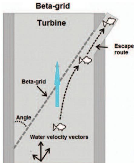
Figure 3. A beta-grid located upstream of the turbine can direct smolts and kelts into the fishway (Calles et al. 2013).
