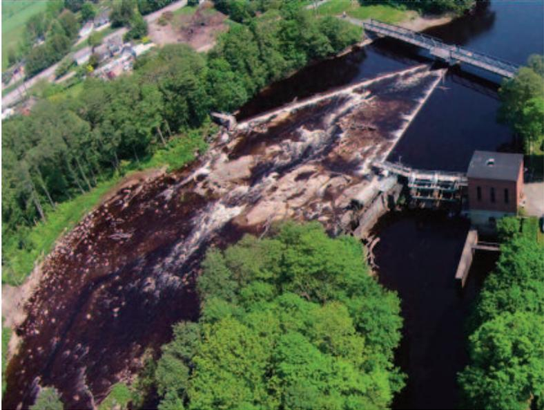
*The dam has been removed (2014) in one of the two main stems in the River Ätran. A construction directs migrating Atlantic salmon into a fish counter situated in the middle of the mainstem.*
