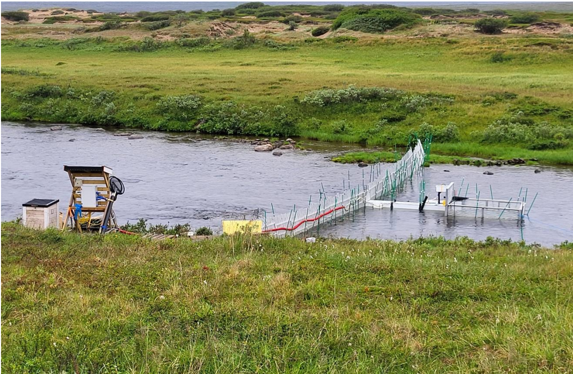
Figure 16. Fence and fish trap on the Skallelva with artificial intelligence prototype to automatically sort pink salmon from Atlantic salmon. Credit: Colin Bean.
