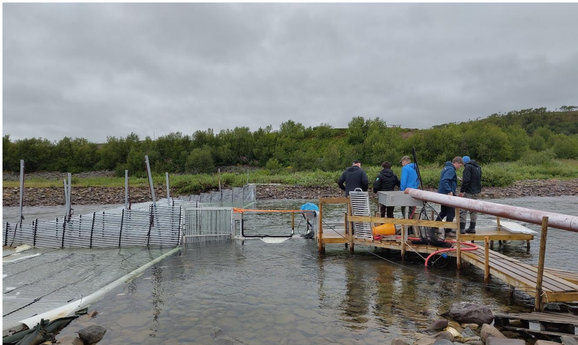
Figure 13. Fish trap on the Vestre Jakobselva, with artificial intelligence prototype to automatically sort pink salmon from Atlantic salmon. Credit: NASCO Secretariat.
