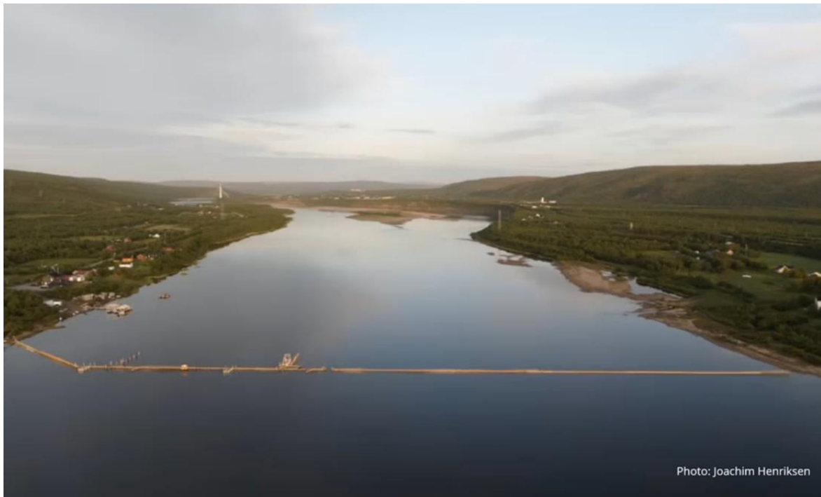
Figure 6. Ariel view by drone of the fence across the whole of the Tanaelva's 400 m width combined with two fish traps. Credit: Joachim Henriksen.
