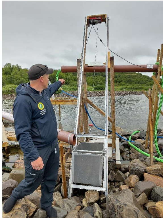
Figure 14. Fish transport system to move pink salmon from trap to fish boxes on the Vestre Jakobselva. Credit: NASCO Secretariat.
